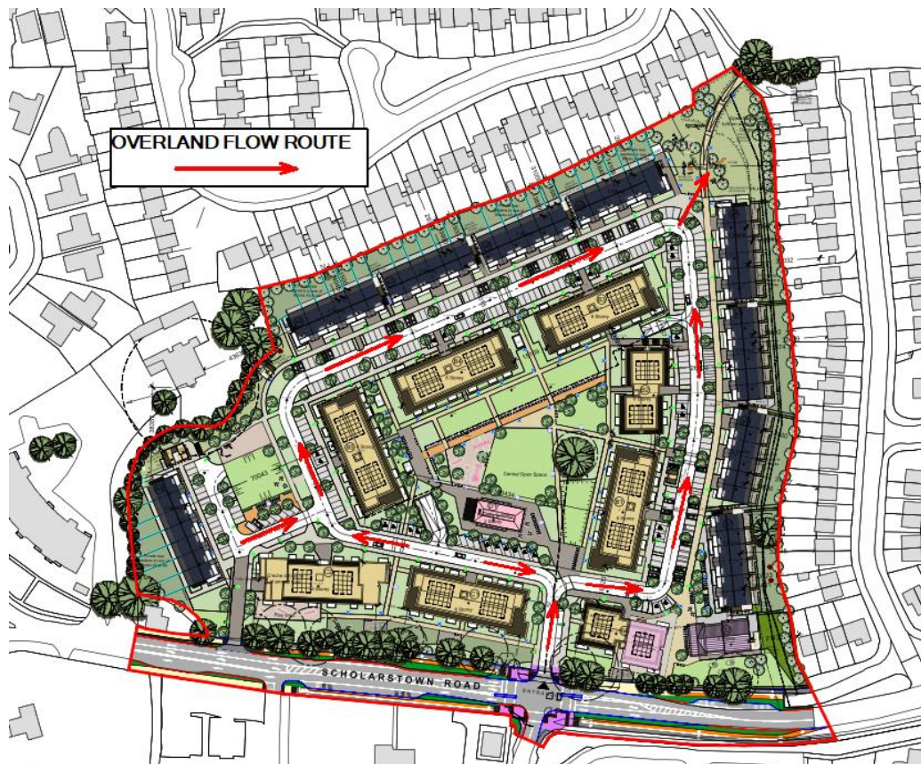
Figure 5.1 – Flood Exceedance (>1%AEP) Overland Flow Routes
